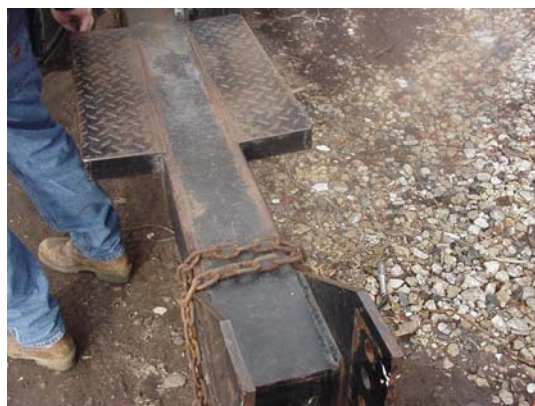
Improperly Modified Yoke
